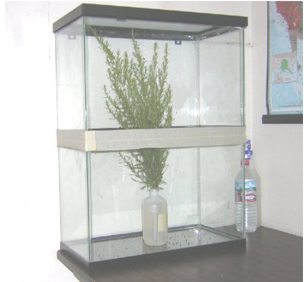
Figure 5. The Open Terrarium Method: With a screen lid, this particular setup consists of 2 ten gallon terrariums taped together (the bottom glass hammered out of one) in order to accommodate taller growing larval foodplants. For most applications, a regular 10 gallon terrarium with screen lid should work fine.
